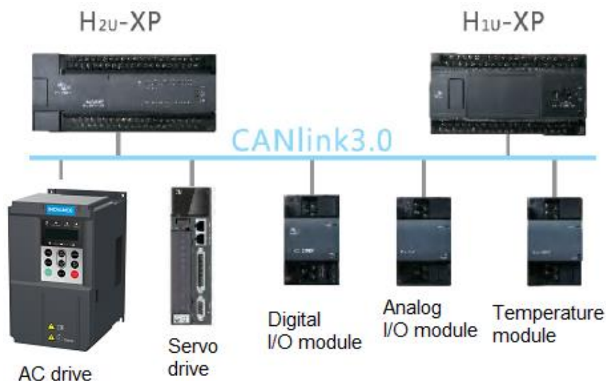
CANlink network topology diagram
